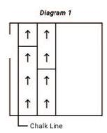
Each Achieve roll will be labeled with a number that corresponds to the sequence in which it came off the machine. It is important to lay the rolls in sequence (roll 1, roll 2, roll 3, etc.) to avoid obvious shade variances.
