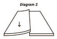
Overlap side edges by 0.125in and force alignment to ensure tight seams.
